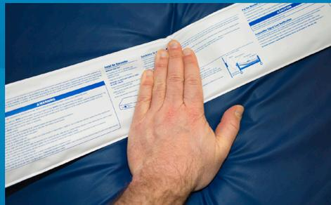
Firmly place pressure on the pad and then release. A long beep from the monitor will indicate it has been synchronized with the pad.
