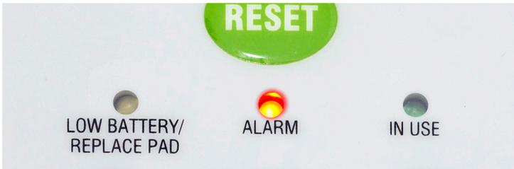
All our monitors clearly show you when they're in use, and when the alarm is going off. You'll also be notified when to replace the batteries and the sensor pad (when using timed sensor pads).
