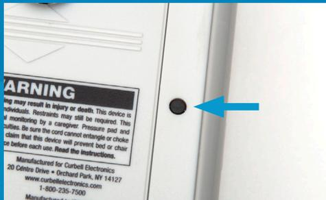
Press and hold the black programming button on the back of the monitor until the monitor beeps three times and the LCD screen displays "PROGRAM MODE".
